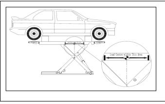
Before entering a car on the lift, make sure that the platforms are at it's lowest position. When placing a car on the lift, the weight must be as centered as possible. Read operating and safety manuals before using the lift. Load vehicle onto the lift using the vehicle lifting guide to determine proper lifting points. Position vehicle over the platforms. NEVER use the lift without placing the rubber bricks between the car and lifting platforms!
